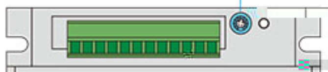
内置调速电位器 RV Built-in speed regulation potentiometer RV
